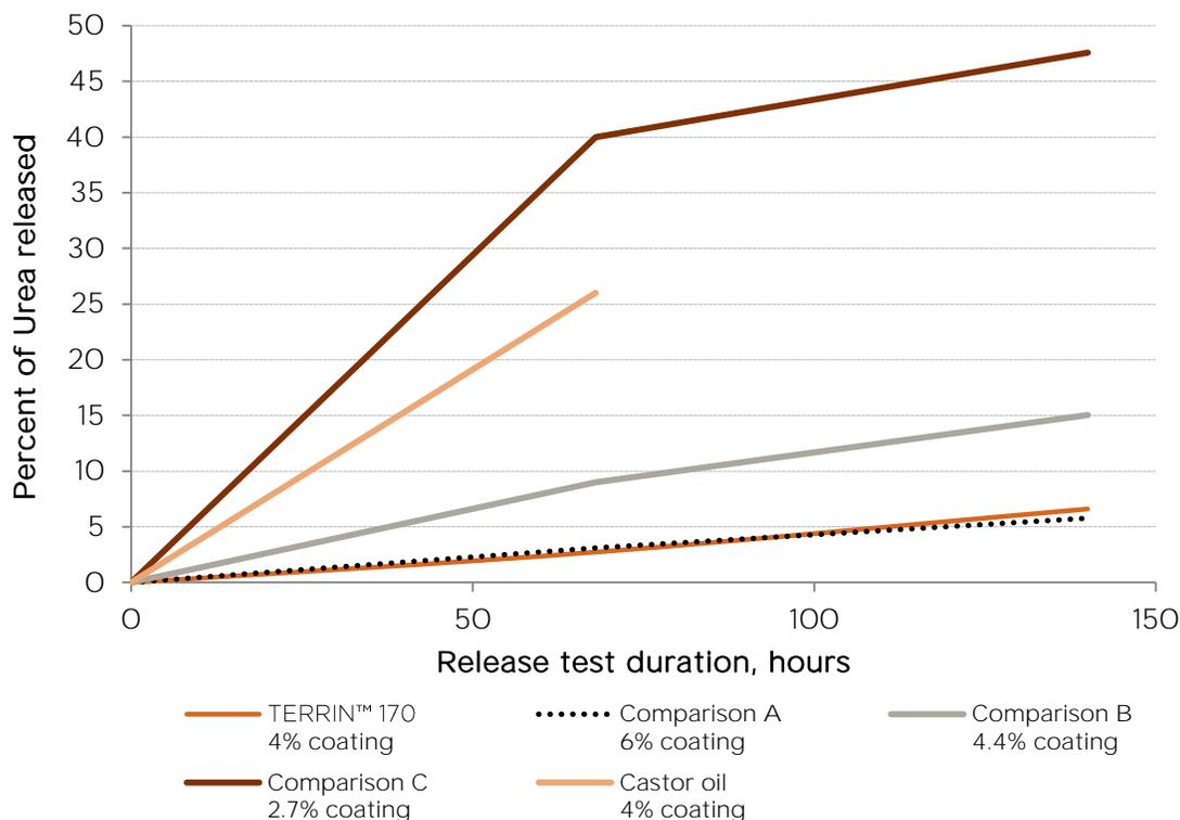
Figure 2: Extended release performance of CRF
